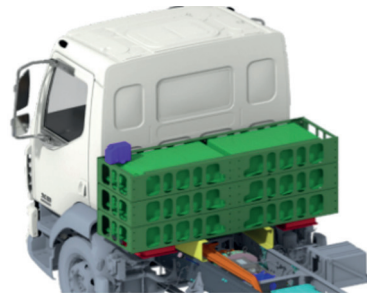
DAF – Battery layout configuration
