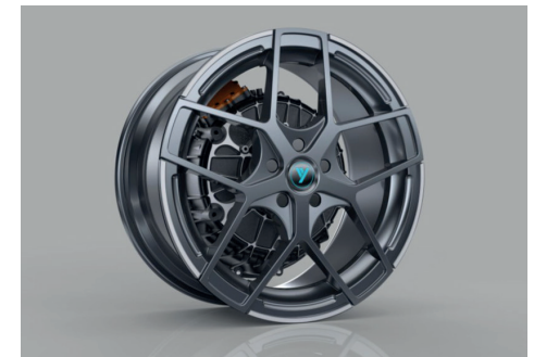
YASA's In-wheel motor can fit an 18 inch wheel
