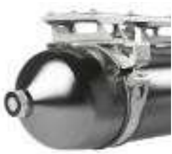
On-board carbon fibre hydrogen pressurised tank, valves and regulators
