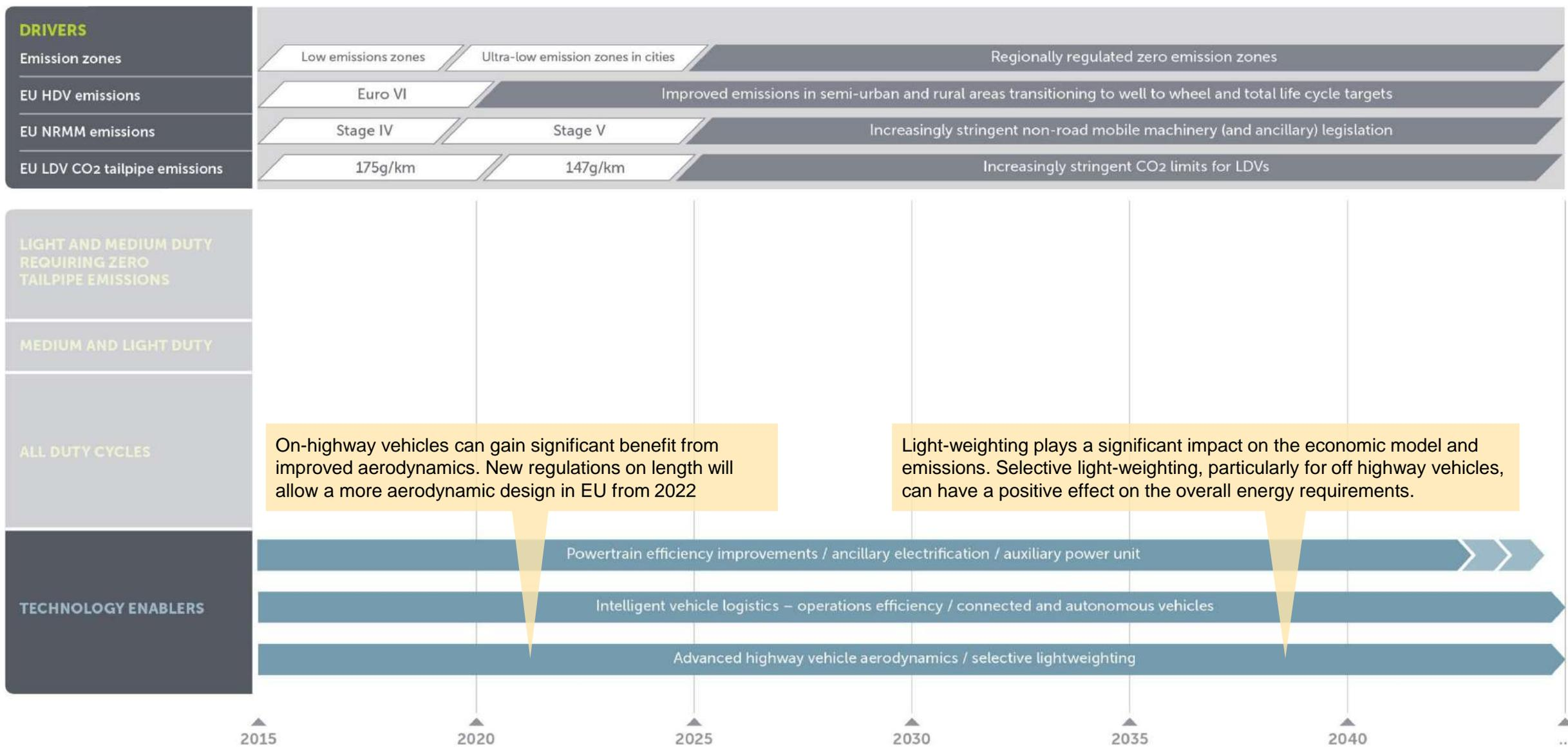
**Technology enablers:** *Improving operational efficiency can lead to significant emissions reduction; connected and autonomous vehicle technology will be a big enabler for fleet wide reductions in CO2 and emissions*
