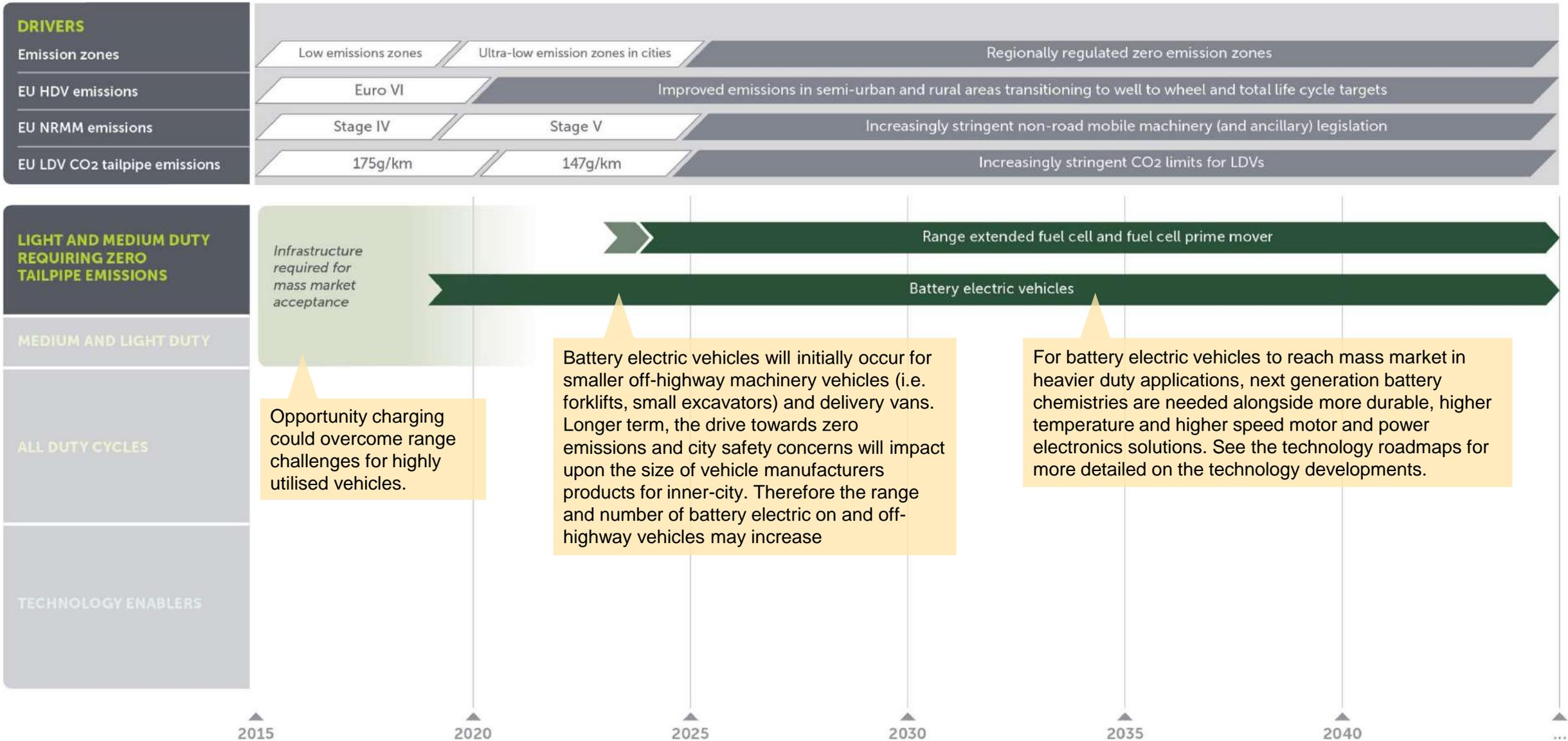
**Zero tailpipe emission:** *The timing of mass market introduction of fuel cell commercial vehicles is uncertain due to lack of infrastructure, however initial uptake could be driven by captive fleets that have a central refuelling location*
